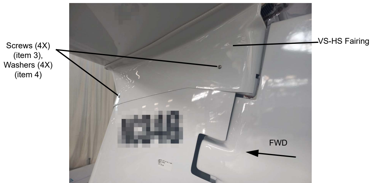
Figure 4. VS-HS fairing installation.
