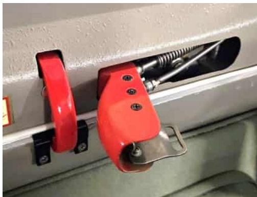
Figure 8. Old door latching mechanism
