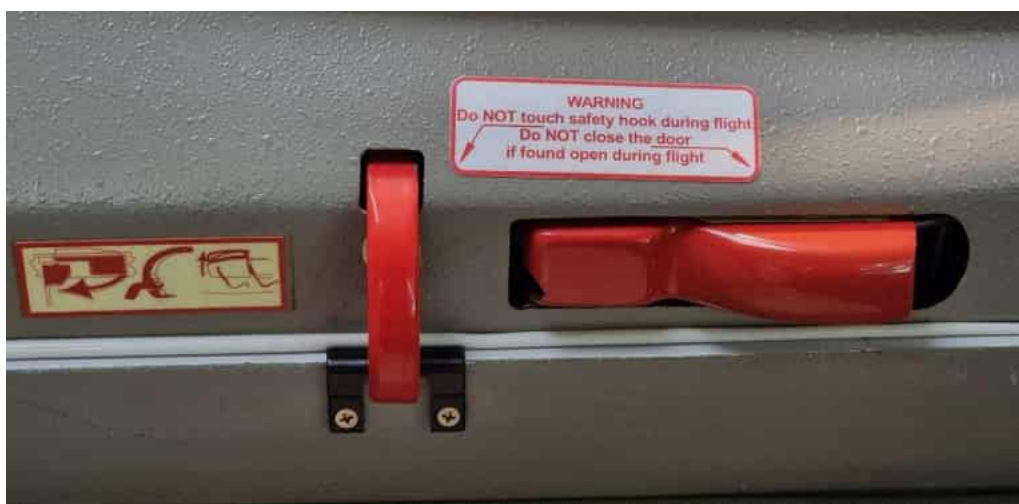
Figure 26. Old latching mechanism (MÄM 40-139 not installed)
