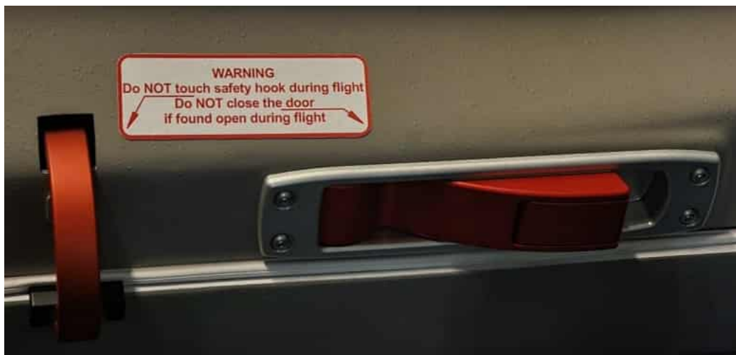
Figure 25. New latching mechanism (MÄM 40-139 installed)
