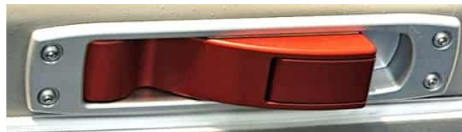
Figure 9. New door latching mechanism (MÄM 40-139 Installed)
