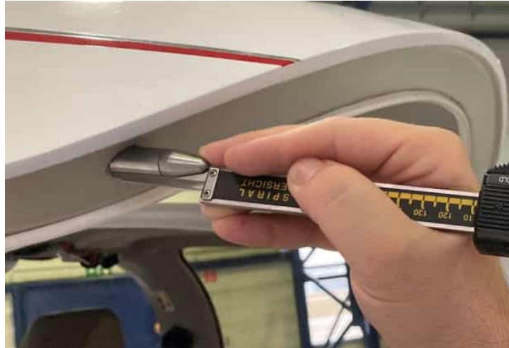
Figure 16. Rear latching bolt
