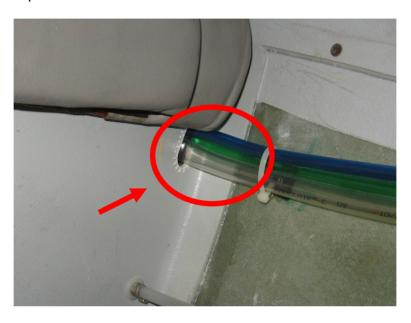
Ensure that any tie wrap bases are secured to the fuselage wall behind the side pocket. If a tie wrap base has been dislodged from the fuselage wall, bond it back into its original position using commercial 5 min Epoxy adhesive.
