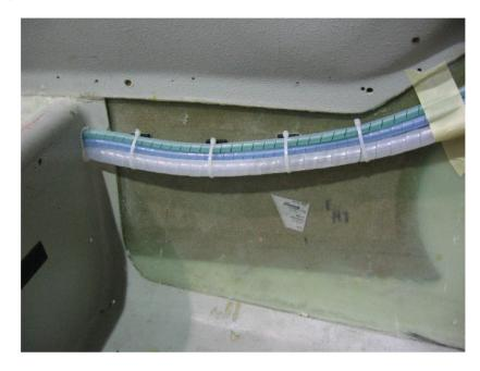
**CAUTION:** Do not overtighten the cable ties to prevent squeezing of the pitot, static and stall warning lines.
