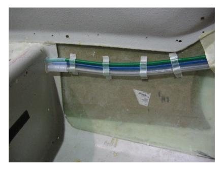
Attach lines to their fittings aft of the floor panel wall. Reinstall all tie wraps removed.
