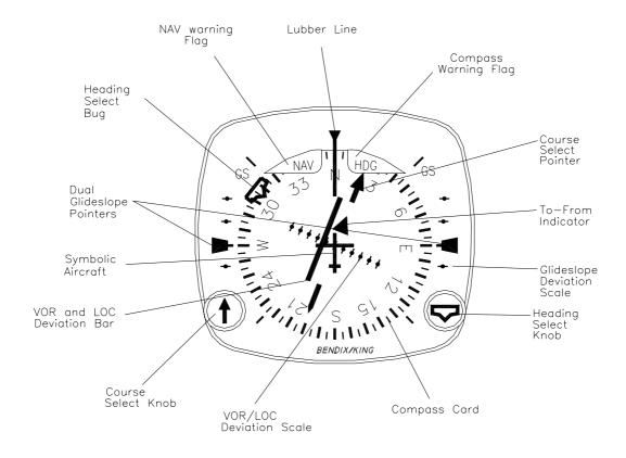
The KI 525A Pictorial Navigation Indicator is the panel display for the KCS 55A Compass System. It replaces the standard Directional Gyro and Course Deviation Indicator (CDI) in the airplane's panel, combining slaved heading and VOR/LOC/Glideslope information into one compact display. By providing a simple, comprehensive visual presentation of the airplanes heading and position in relation to a desired course, the pilot's navigation workload is considerably reduced.
