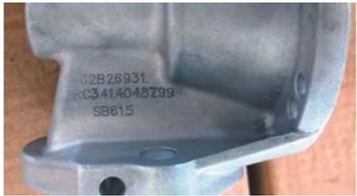
Figure 1 Date Stamp Code with “SB615” on Fuel Pump Web
