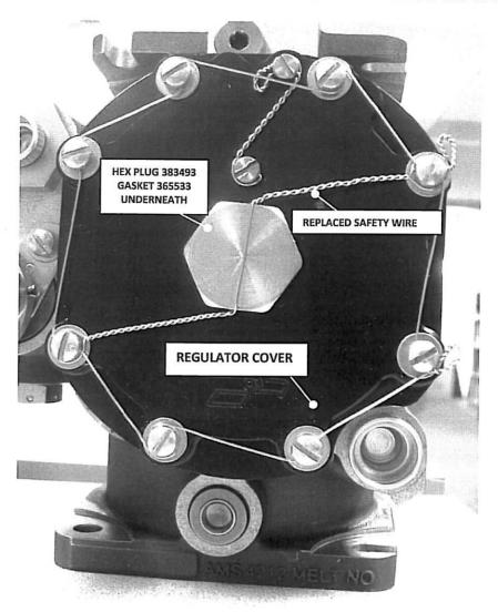
Note: Plug safety wire is wrapped around regulator screws under existing wire. It does not go through the holes in the screws.
