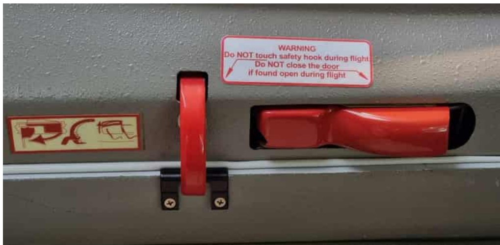
Figure 26. Old latching mechanism (MÄM 40-139 not installed)
