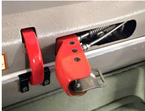
Figure 8. Old door latching mechanism
