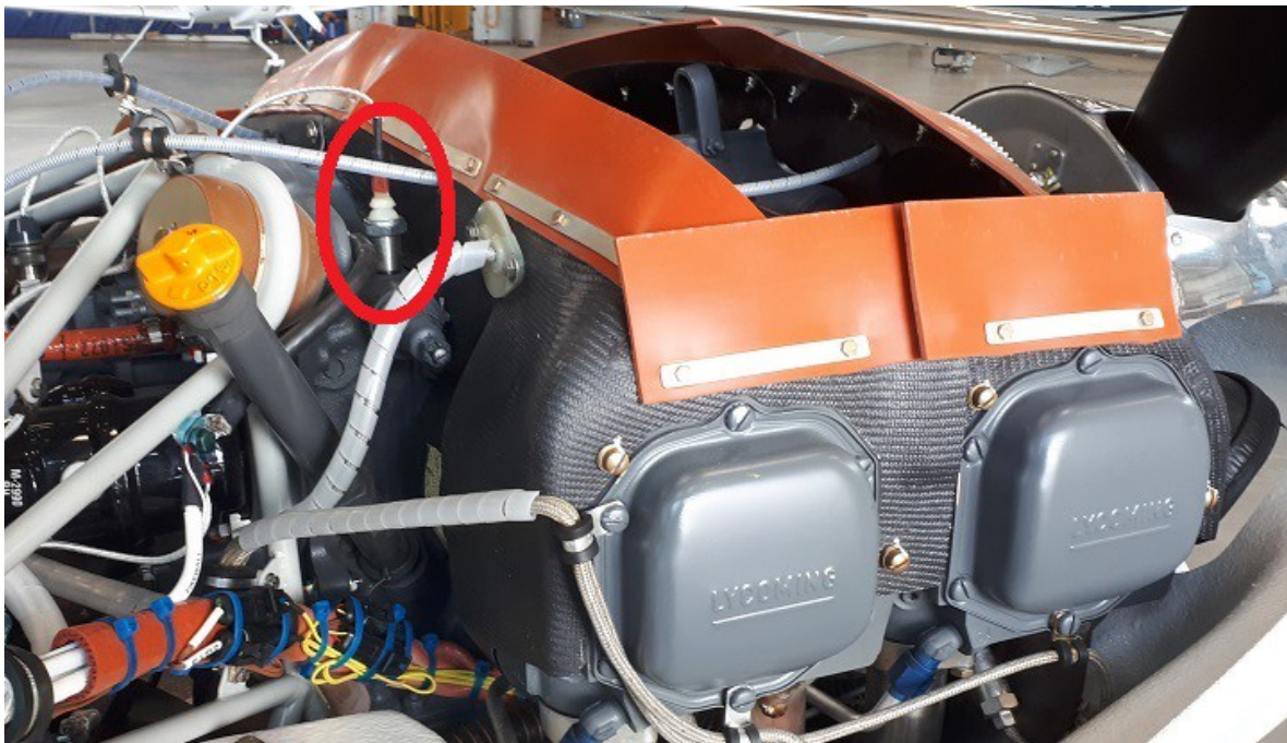
Figure 1. Original oil pressure switch installation.
