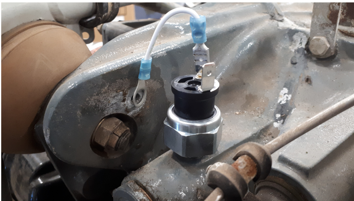
Figure 2. New oil pressure switch (item 1) with bonding wire (item 2). Wire harness from aircraft not shown.
