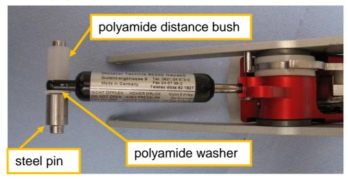
Install the new steel pin with the polyamide washer and the polyamide distance bush to the door handle mechanism frame:
