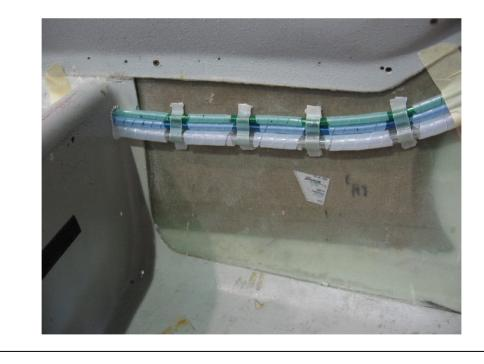
Attach lines to their fittings aft of the floor panel wall. Reinstall all tie wraps removed.
