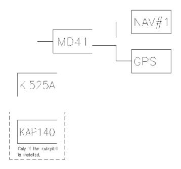
Either the NAV #1 (VOR) information or the GPS information can be switched to the data inputs of the HSI KI 525A. In addition, this navigation information is also used for the KAP 140 autopilot, if the autopilot is installed.
