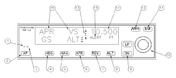
1. PITCH AXIS, (P) ANNUNCIATOR - When illuminated, it indicates failure of the pitch axis and will either disengage the autopilot or does not allow engagement of the pitch axis. The P light may illuminate with the autopilot disengaged. This condition can occur during maneuvering flight when g thresholds are exceeded. The autopilot monitor will not allow engagement during illumination.
