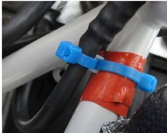
Figure 3. Safety rope at aft right of the engine. Note the silicone tape, spacer, and two zip ties used to secure the safety rope.
