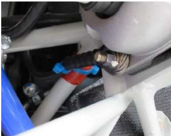
Figure 3. Safety rope at aft right of the engine. Note the silicone tape, spacer, and two zip ties used to secure the safety rope.
