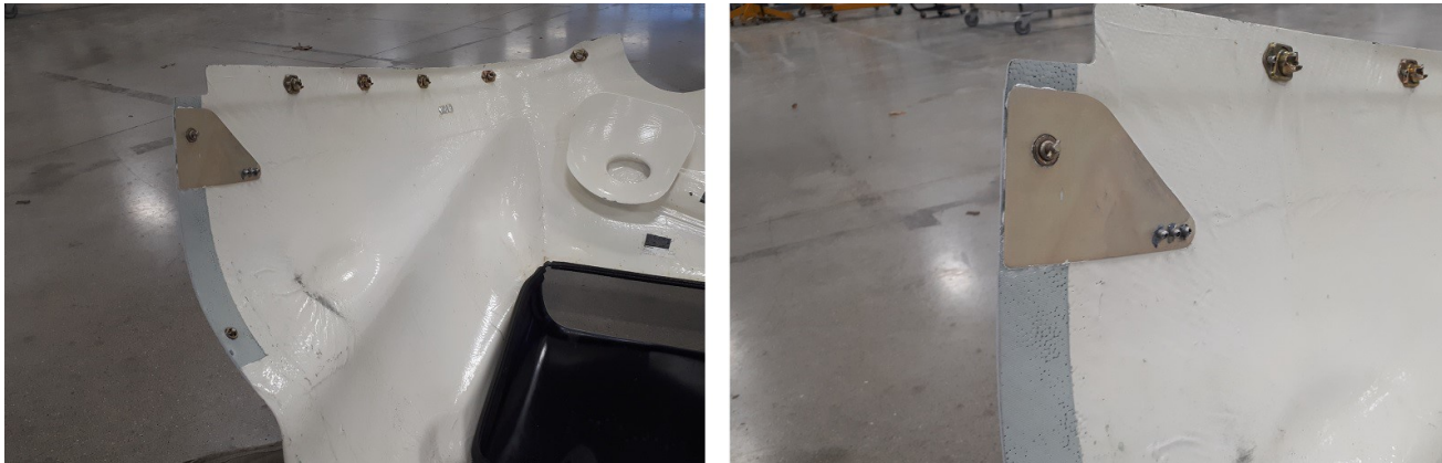
Figure 1. Left: position of item 1 on the left-hand side of the lower cowling. Right: zoomed view. Not shown: apply Nycote to the rivet shanks on the inside of the cowling after the sealant has cured (step 22).
