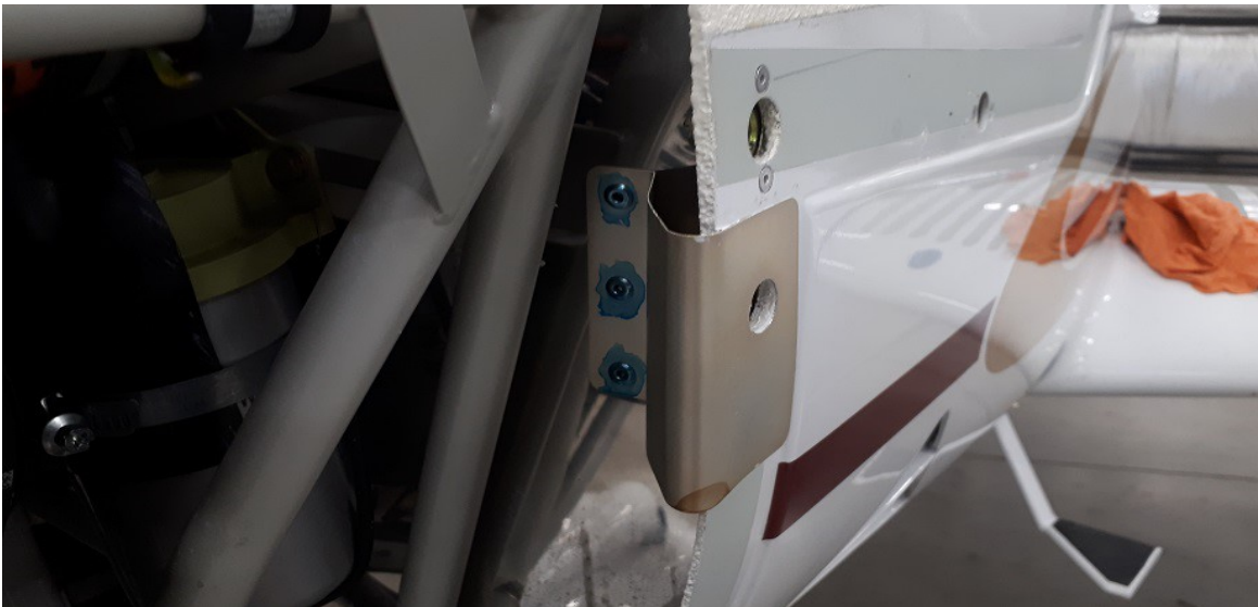
Figure 2. Position of item 3 on the left-hand side of the aircraft. Not shown: also apply Nycote around the edges of item 3 where it contacts the firewall (step 30).
