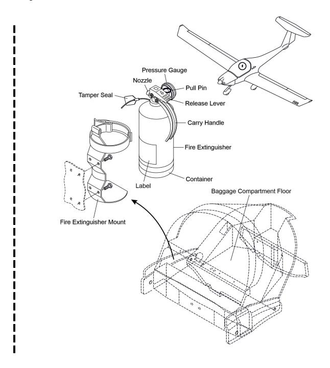
Figure 1: Fire Extinguisher Installation
