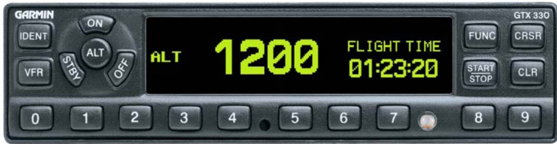
Figure 2: GTX 328/330 Transponder Front Panel
