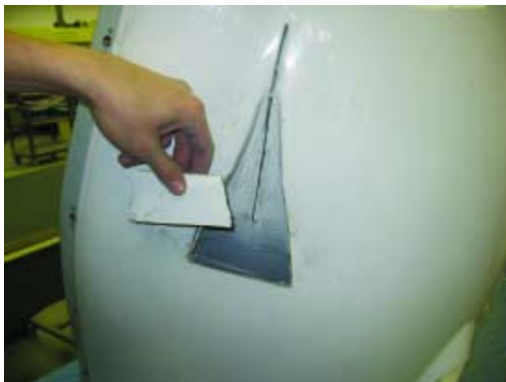
Figure 7 - Removal of the NACA Aft Lip
