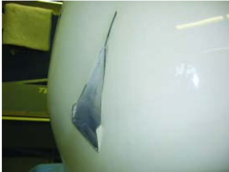
Figure 8 - Trim Flush with the Surface of the Cowl
