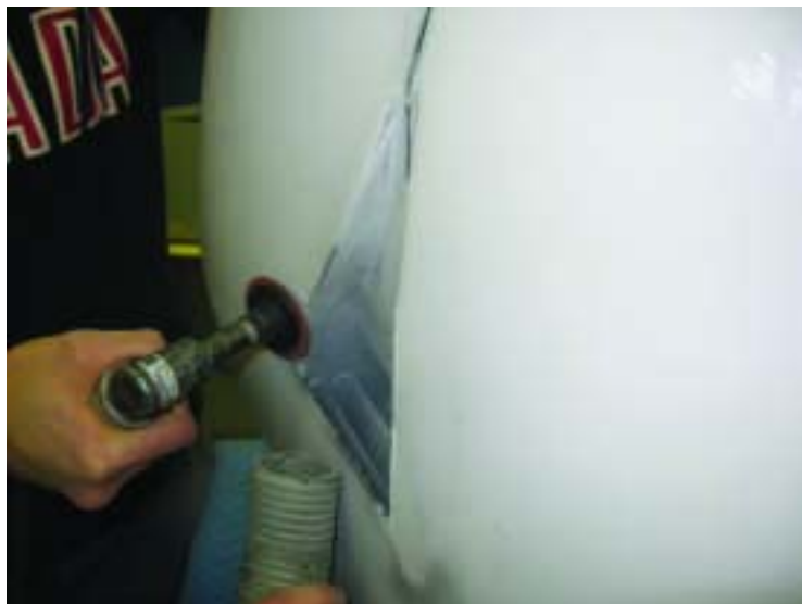
Figure 9 - Trim Flush with the Surface of the Cowl
