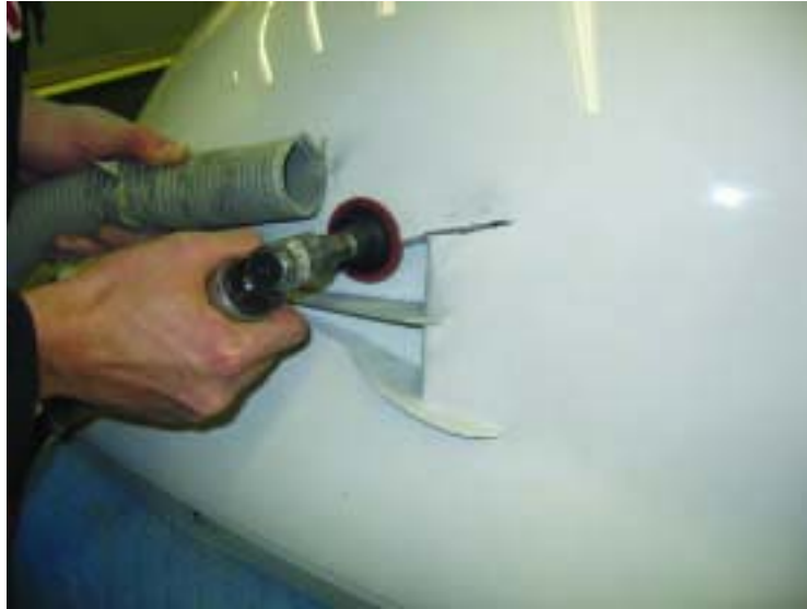
Figure 2 - NACA Duct Ramp Surface
