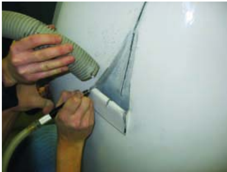
Figure 6 - Removal of the NACA Aft Lip
