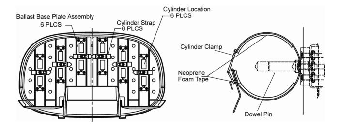
Ballast Mounting Brackets and Cylindrical Ballast Clamps
