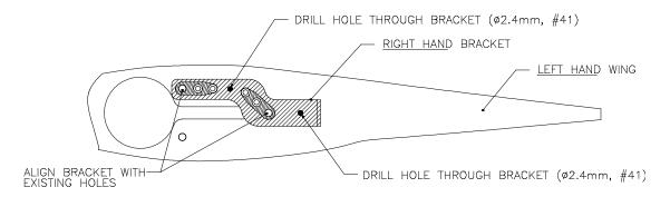
5. Align nut plate (item 12) on left hand wing as shown, and mark the rivet locations with a permanent marker. Remove nut plate, and drill.
