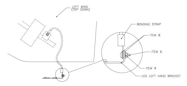
9. Apply surface protection (Nycote 7-11 or equivalent) to bonding connection.
