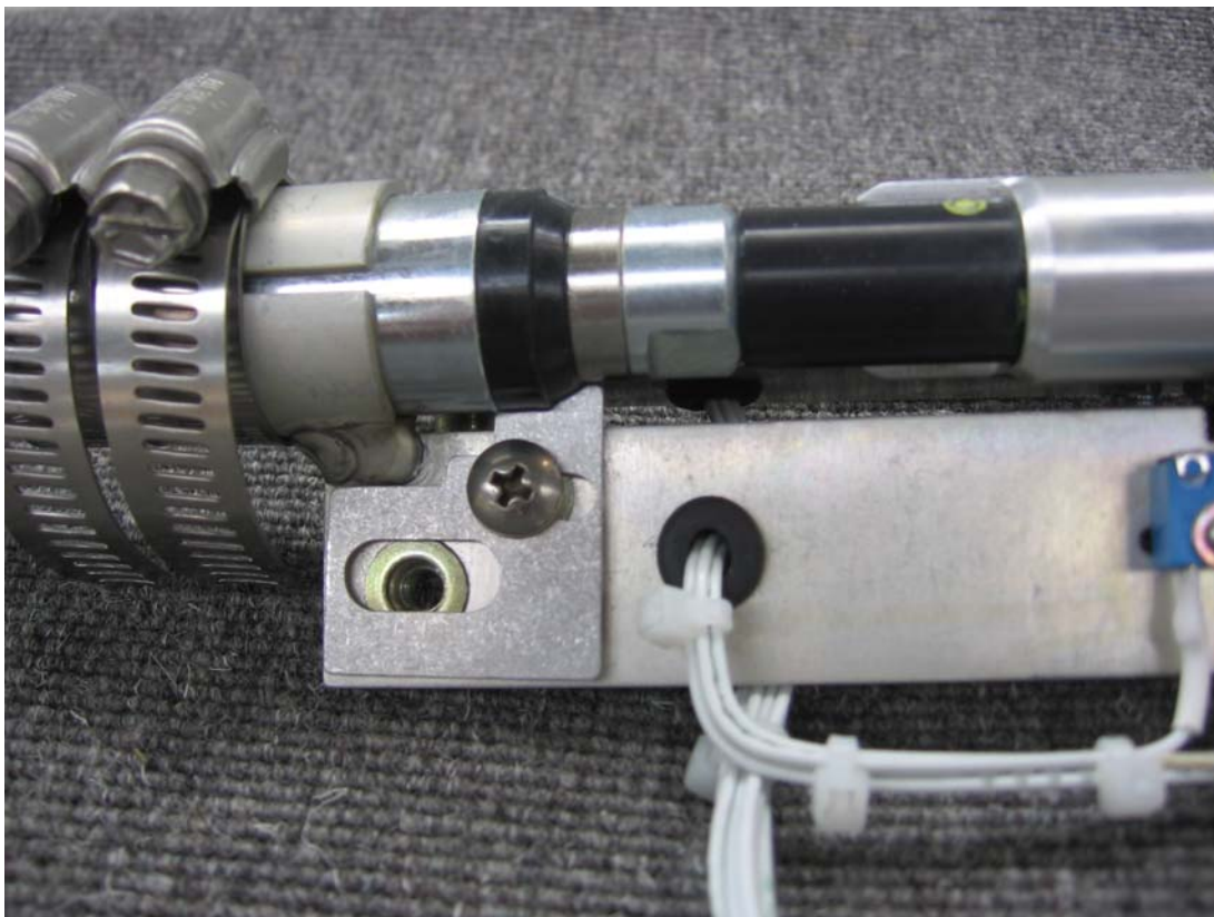
Figure 2 – Seal Retainer Installation (Switch Cover Removed for Clarity)
