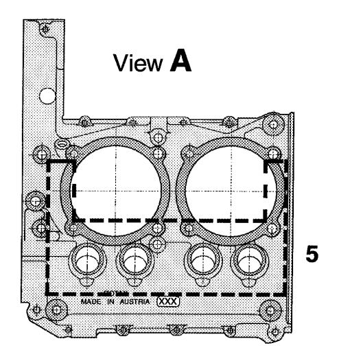
Figure 2. Engine Crankcase Inspection Areas – View A
