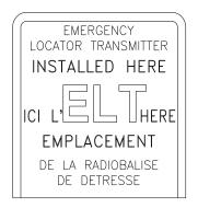
34. On fuselage underside (belly), by left wing
